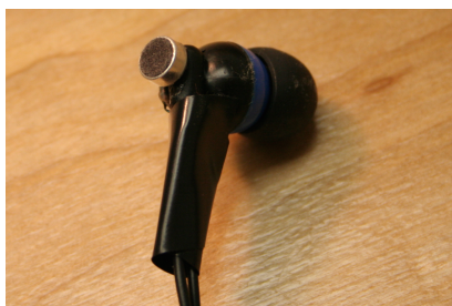
Figure 2: Earbud modified to record audio from two mics, one inside the earbud and one attached to the back (shown).
