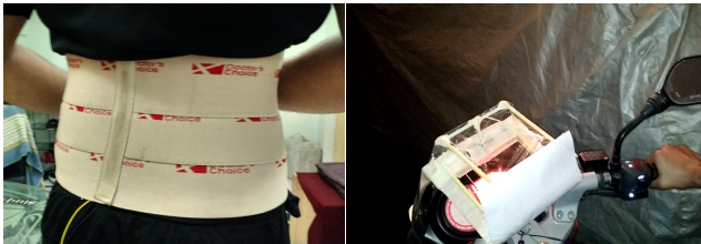
Figure 1: Left: Belt embedded with Flex sensor. Right: Mechanically Moving Display on the Speedometer
