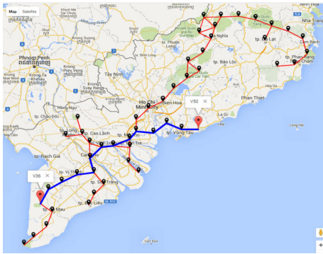
Figure 11. The shortest path for data dissemination from node v_{50} to gateway node v_{36} .
