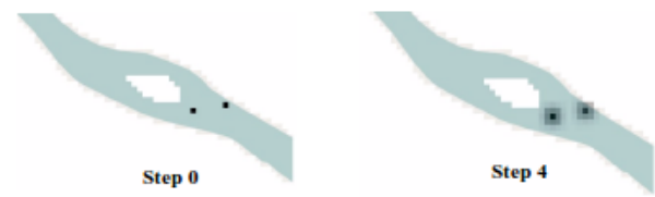
Figure 14. The parallel simulation of diffusing pollution in a river. This is initialized with two polluted points (dark points).
