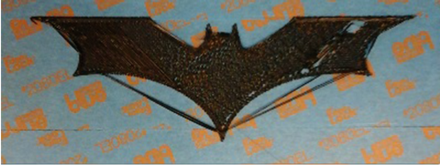
Fig. 2. The beginning of a failed print. Internal error caused by PLA not sticking to the printerbed, and external error caused by PLA not sticking to the previous layer.
