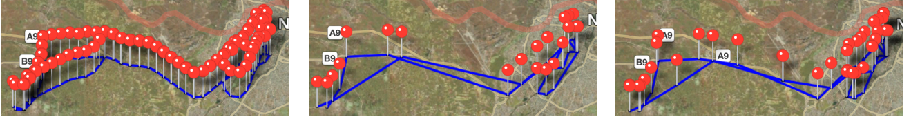
Figure 1: Trajectory tracking examples. Left: GPS service using distanceFilter=500m. Middle: SLU service. Right: Proposed approach that combines both services.
