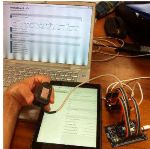
Figure 2 – Sample setup showing the heart rate being acquired and visualized in real-time on the web.
