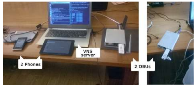
Figure 3. Setup used for tests. Two OBUs with one mobile device connected to each one and a computer running as the VNS server and sharing Internet connection to the OBU.
