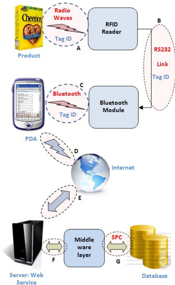
Figure 4: Accessible caption: The figure shows the complete data flow model for the proposed system. Product, RFID reader, Bluetooth module, PDA, store server and database are shown in a linear data flow model as explained in the Section 5.
