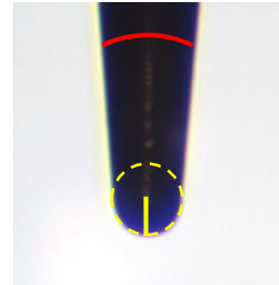
Fig. 1. The solid lines with red and yellow are angle and radius of a LED probe, respectively.
