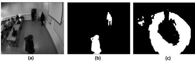
Figure 7. (a). Input Video (b). Frame difference (c). Frame accumulation
