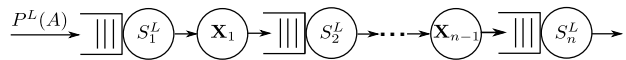
Figure 2: A network model consisting of packetized arrivals, services and packet scaling elements.
