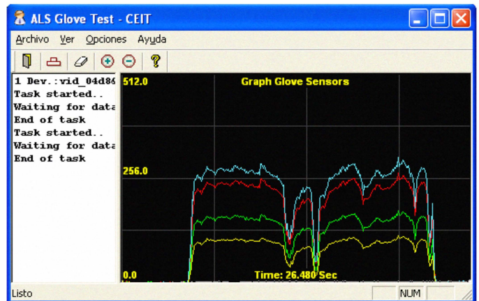
Figure 8. PC application showing hand-grip force test results.
