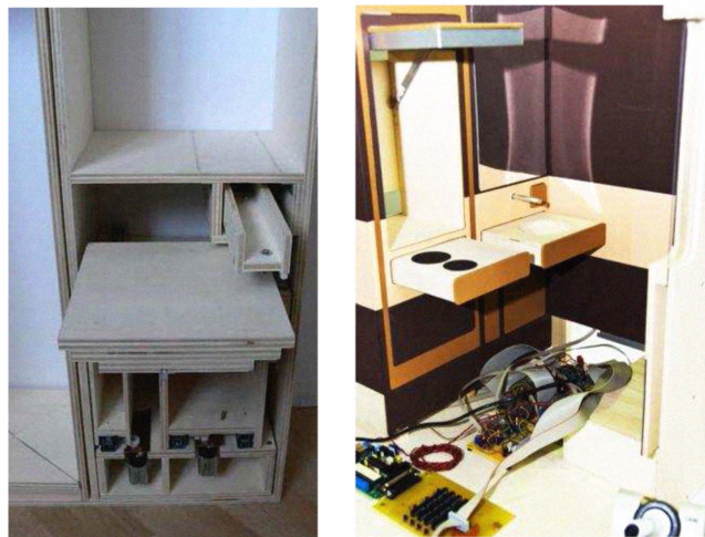
Figure 7. Left: 1:1 model of a Service Core “chassis”, customizable through modular and compatible sets of functionalities, smart appliances, sensors, actors, design fit outs. All functions can be automatically retracted into the core unit. Right: Sensor and actuator-equipped scale model of a service core with a model kitchen compartment (left) and hygiene area with functional water supply and sink (right).
