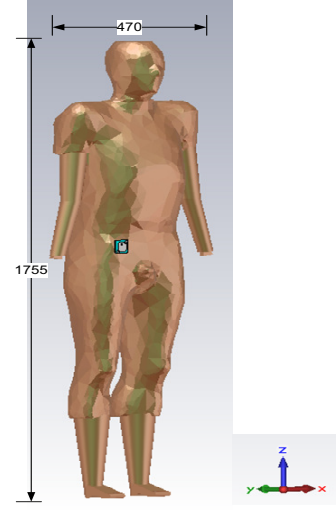
Fig. 2. Structure of realistic high-resolution numerical model of the human body (all lengths are in mm)
