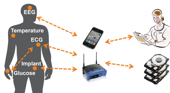
Figure 1: A typical BAN with sensors monitoring vital health signals and transmitting them through intermediate devices to destinations for assessment and storage.
