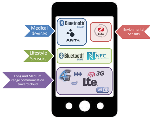
Figure 3: Communication interfaces supported by the smartphone centric application.
