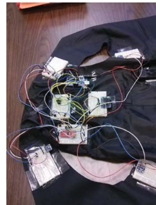
Figure 5. Image of LightVest laid out flat, with light sensors at the four outside corners, Arduino Uno at middle top, OLED display at middle right, central hub breadboard at middle right, and multiplexer at middle bottom.
