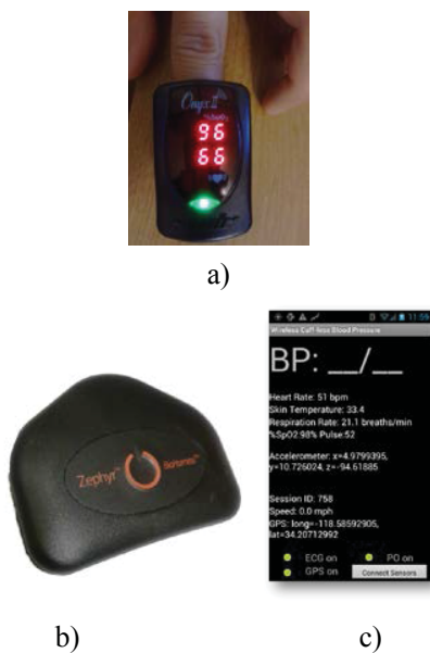
Figure 3. Virtual Cuff Sensor and Interface. a) Nonin Onyx II 9560 Fingertip Pulse Oximeter used on the finger to derive PPG signals. b) Zephyr Bioharness strapped to the users chest collects ECG data. c) Screen Shot of Android App
