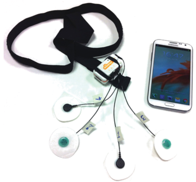
Figure 2: Wearable 4 leads ECG sensor (using Shimmer2R node) and the smartphone used to collect data.
