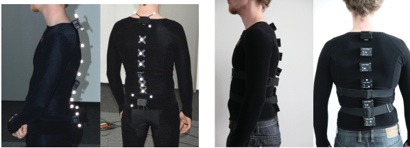
Figure 3: Experimental setups: Precision setup with markers for optical reference (left) and approximation validation with 9 IMUs (right).
