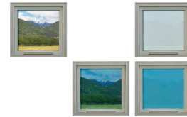
Figure 3. End-states of the windowpanes. a. PDLC layer is active and electrochromic is inactive; b. PDLC and electrochromic layers are inactive; c. PDLC and electrochromic layers are active; d. PDLC layer is inactive and electrochromic is active.
