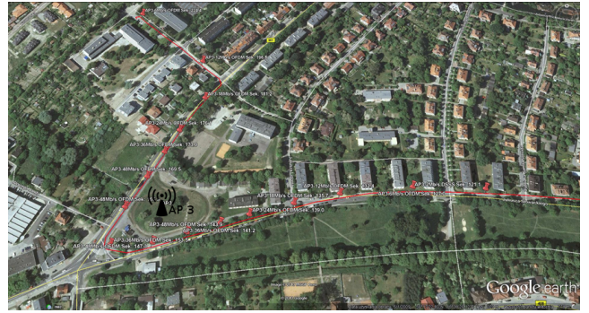
Figure 3: Map of simulated AP with marked path and point at which coding rate changes.
