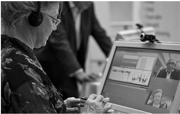
Figure 1 - The ViewCare telemedicine solution supports a video based secure connection to be established. Also, it allows data to be exchanged from connected devices; a cabled blood pressure device and a cabled glucometer.
