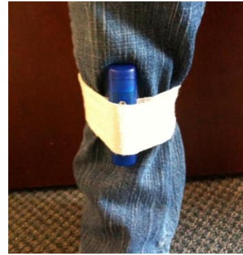
Figure 1. The accelerometer mounted on the leg (The z axis of the accelerometer is perpendicular to the surface of the leg)
