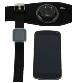
Figure 1: The apparatus: Zephyr BioHarness 3 (top), Sony SmartWatch (left) and LG Nexus 4 (right).
