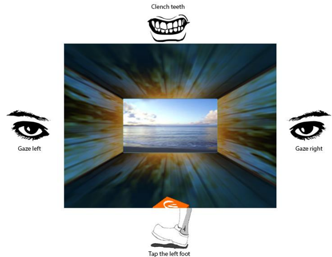
Figure 1. An illustration of the control paradigm. In this example the user is successfully replicating the drop command by tapping their left foot.
