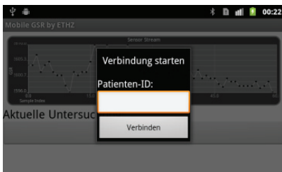
Figure 1: Android Application asks for the patient ID to issue the connection to the sensor device. The real-time annotation functionality also works when the Bluetooth connection between phone and sensor is lost or terminated. The annotations and sensor data is merged afterwards.
