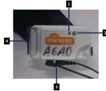
Figure 2: Sensor node with reset button (1), status LED (2), Connectors for GSR electrodes (3), holder and Velcro strap (4).
