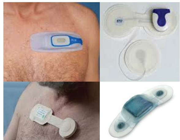
Figure 2. Wearable patch ECG monitor. Top-L: NUVANT [11]. Top-R: V-Patch [12]. Bottom-L: HRV011 [9]. Bottom-R: Zio Patch [10]
