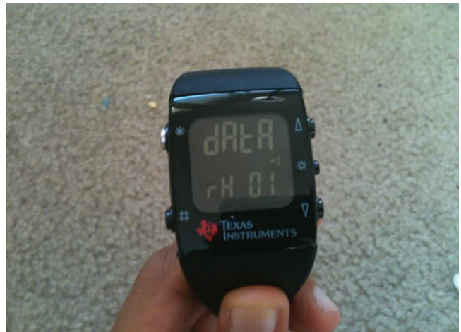
Figure 9 Data received on the nurse's watch notifying the fallen node number - node 1
