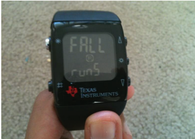
Figure 8 "Fall" signal on the patient's watch -programmed as node1
