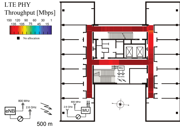
Fig. 3. In-building coverage with cognitive repeater deployment
