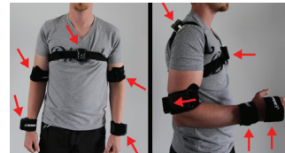
Figure 3: Two setups used for evaluating the tracking precision: upper body (left) and full arm (right). The red arrows mark the IMU positions.
