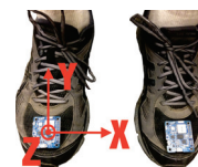
Figure 1: Sensor mounting position on the shoe.
