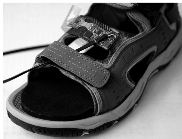
Figure 3 During test measurements, the capacitive insole sensor was placed in a sandal with read-out electronics.
