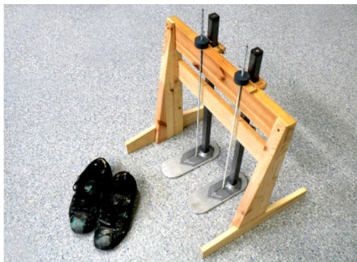
Figure 2 The Human body phantom with adjustable legs. European foot size is 41. Leg to leg Impedance is 500 Ω. Test shoes used in the tests had 15 mm thick synthetic rubber soles. Sensor array is under a plastic floor covering.
