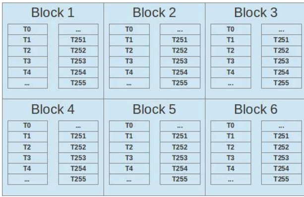
Figure 2: Here is a grid of thread blocks. Each block is configured with 256 threads. The kernel code associated with these blocks will be executed 1,536 (6 x 256) times.
