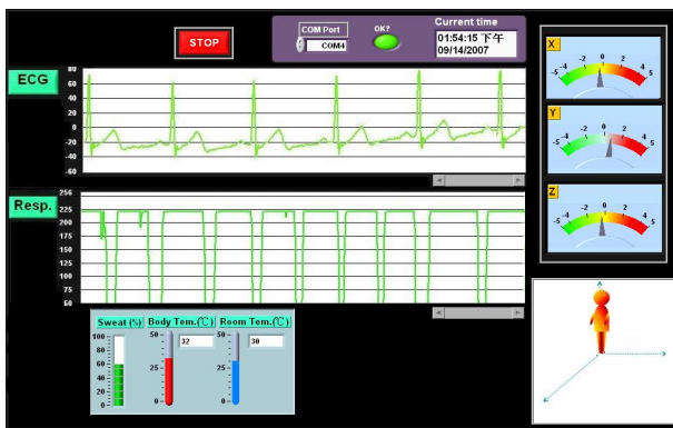
Fig. 2. The LabVIEW interface of the remote computer for typical measured data
